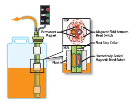
The switch actuation may be used for alarm, solenoid, pump or other fluid control operations.
